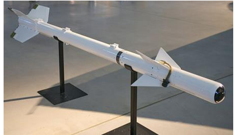
K-13: Short-range, infrared homing air-to-air missile developed by the Soviet Union
