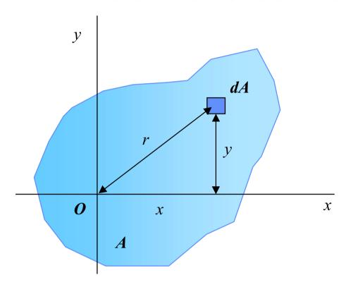
The *polar moment of inertia of*an area A with respect to the pole
