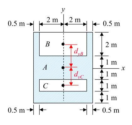
$$I_{x} = (\overline{I}_{x} + Ad_{y}^{2})_{A5 \times 6} - (\overline{I}_{x} + Ad_{y}^{2})_{B4 \times 2} - (\overline{I}_{x} + Ad_{y}^{2})_{C4 \times 4}$$
