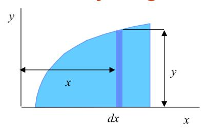
The rectangular moments of inertia  $I_x$  and  $I_y$  of an area are defined as
