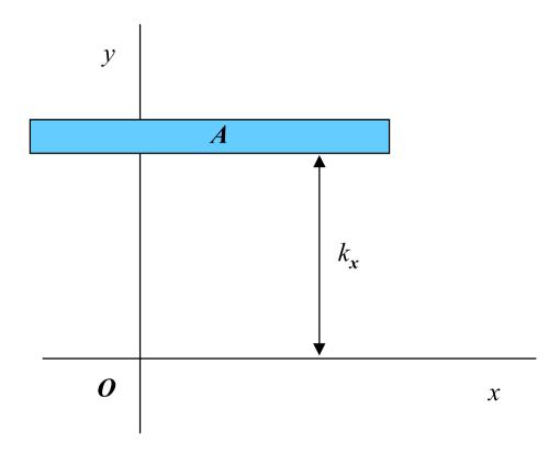
The *radius of gyration of an area* A with respect to the x axis is defined as the distance  $k_x$ , where  $I_x = k_x A$ . With similar definitions for the radii of gyration of A with respect to the y axis and with respect to O, we have
