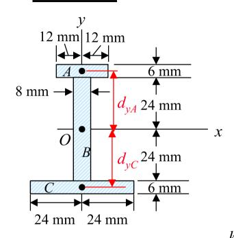
$$I_{x} = (\overline{I}_{x} + Ad_{y}^{2})_{A} + (\overline{I}_{x} + Ad_{y}^{2})_{B} + (\overline{I}_{x} + Ad_{y}^{2})_{C}$$
