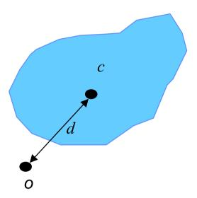
A similar theorem can be used with the polar moment of inertia. The polar moment of inertia  $\overline{J_o}$  of an area about O and the polar moment of inertia  $J_C$  of the area about its
